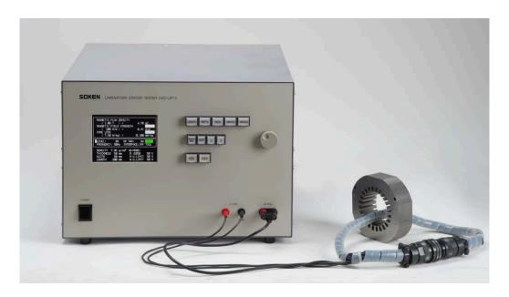
DAC-LST-3 is designed for a pass/fail judgment test of lamination stators of motors by comparison with a reference (\*).
